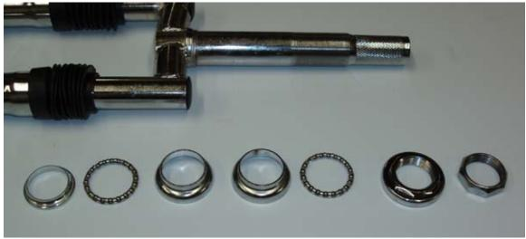
Order: Bearing Ring, Bearing, Bottom Cup, Scooter Goose Neck, Top Cup, Bearing, Bearing Nut Cup, Lock Nut.
